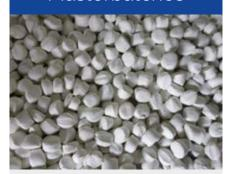
We make polymer specific masterbatches with various loadings of Titanium Dioxide (TiO2) for maximum whiteness index, dispersion and desired opacity of a product.
